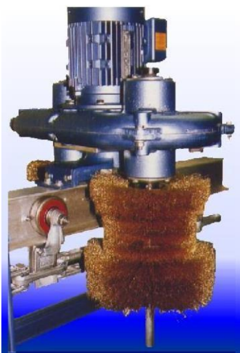
OP-8 conveyor chains and equipment for cleaning of bearing drums
