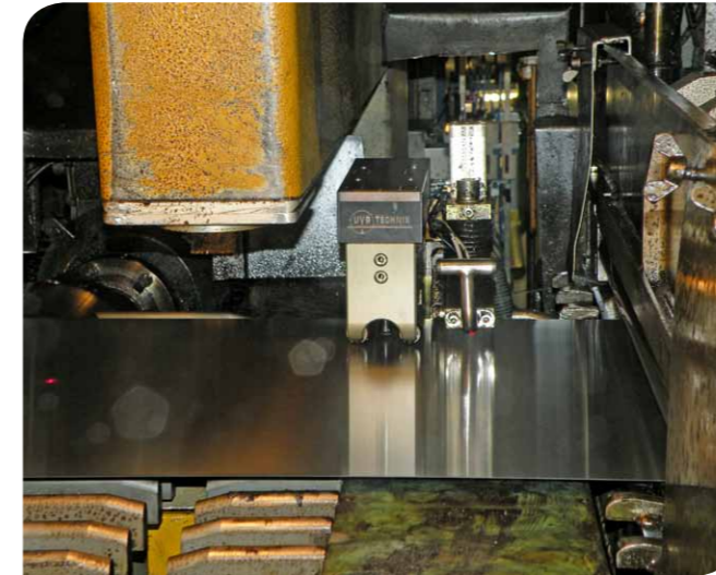
C.D. Waelzholz (werk Wickede), Germany, bimetals, cold rolling mill - Contact thickness gauge used for on-line calibration of X-ray gauge
