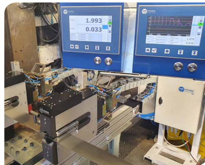
Tenneco, Italy, bimetals, rolling mill - Single line gauge + scanning head
